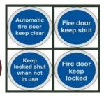
These will either be 30 or 60minute fire protected doors, the 60minute doors are located on the perimeter of the fire zones. All fire doors are identified with signage. When closed into the door frame, these doors will provide protection against fire and heat for the time stated. Fire doors should never be held open with wedges as they could help fire and smoke spread quicker.
