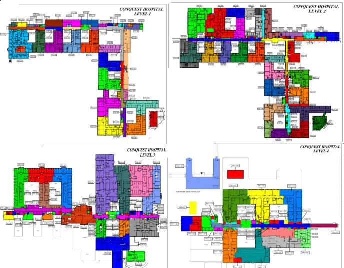
Each different fire zone is identified with a different colour. The fire zones are separate areas which are protected with 60minute fire protective materials (e.g. fire walls, fire doors etc), allowing people to evacuate from a fire affected zone into a safer area of the hospital.
