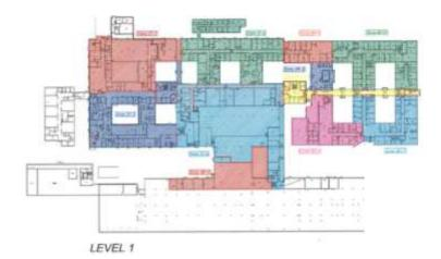
Each different fire zone is identified with a different colour. The fire zones are separate areas which are protected with 60minute fire protective materials (e.g. fire walls, fire doors etc), allowing people to evacuate from a fire affected zone into a safer area of the hospital.
